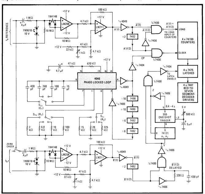
**Angular accuracy.** Meter utilizes tracking ability of PLL to perform phase measurements accurate to 0.1°. 4046 delivers clock signal equal to 3,600  $f_a$  to conventional display (not shown), where count time is determined by  $f_b$ . Thus phase angle of  $f_b$  with respect to  $f_a$  is displayed.
